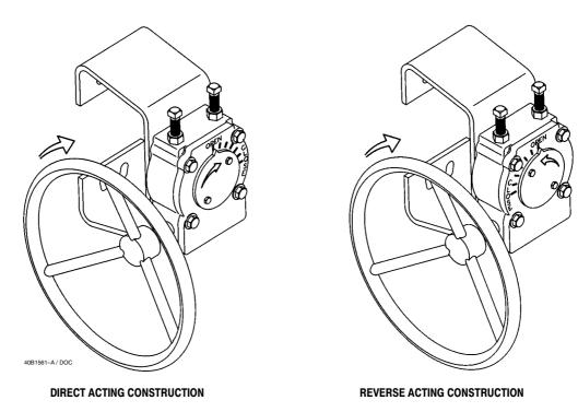
Figure 2. Direct and Reverse Acting Actuator Constructions
